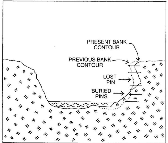
Bank erosion pins and placement
