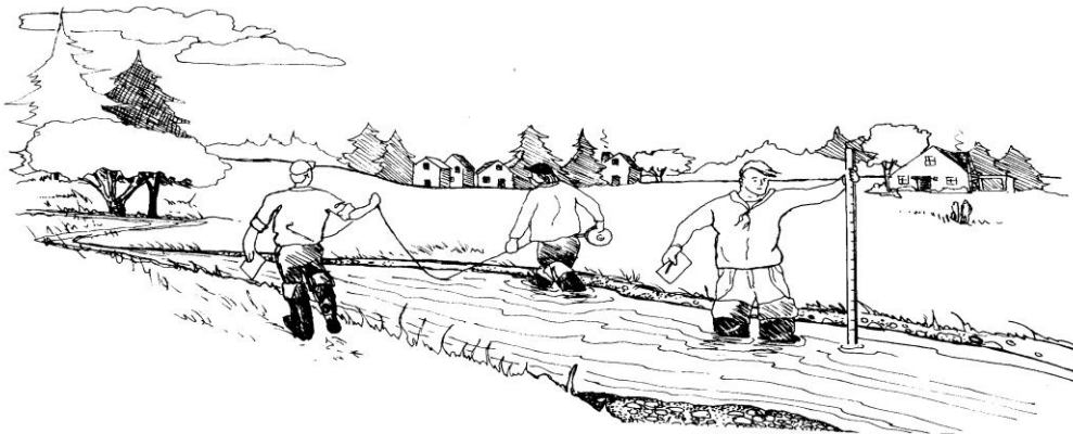
Figure 3.3. Preparing to measure channel cross section
