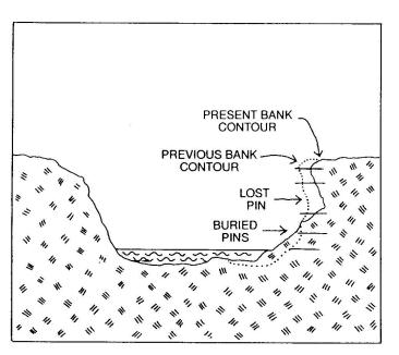
Bank erosion pins and placement
