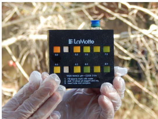
Figure 4: Determining the pH of the stream water. Note the blue capped tube that is being compared to the colored squares.
