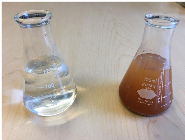
Figure 6: Showing the turbidity of water. The jar on the right is much more turbid than the jar on the left.
