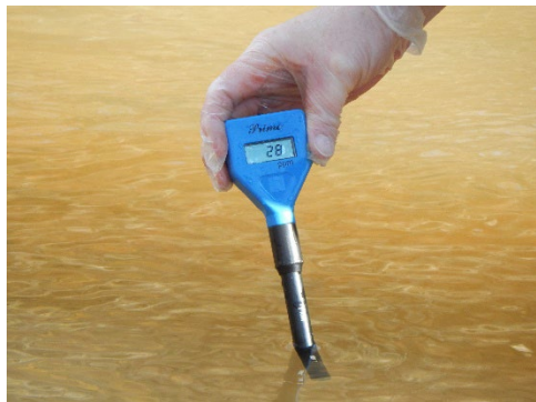
Figure 3: Citizen scientist measuring conductivity in a stream.
