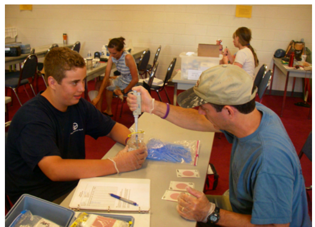
The Olive family team Justin and Robert, pipette an E. coli sample onto Petrifilm growth plates.
