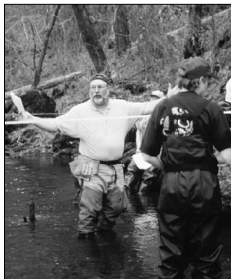
At a recent workshop Ted demonstrates taking cross-section measurements.
