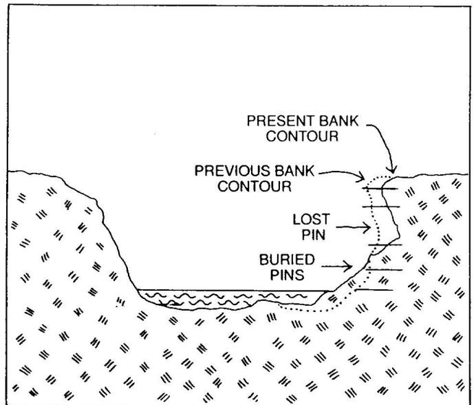
Bank erosion pins and placement
