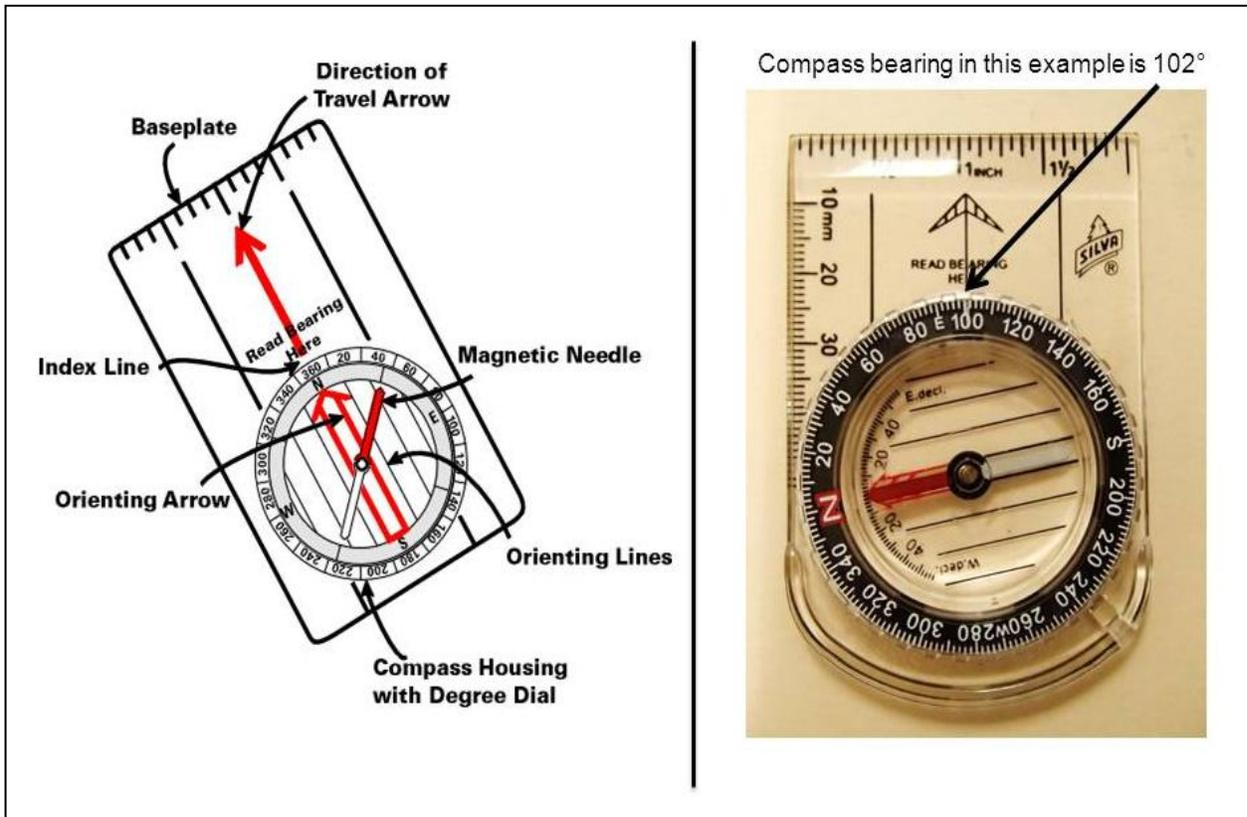
Figure 3.1 How to Take a Compass Bearing
